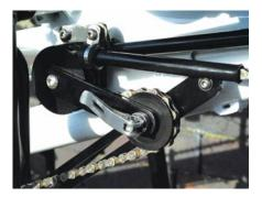
This chain tensioner enables the front boom to be moved in or out to accommodate different sizes of stoker
