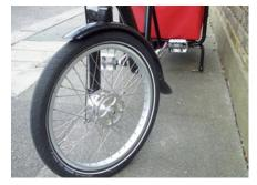
(Above) The 8Freight's hubs are supported on one side only. Puncture repairs are easy, upgrades less so
