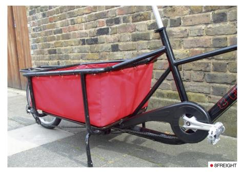
brake hubs are part of the frame, so there's no need for torque arms to brace them.
