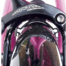
(Above) Good clearance under the brake calliper is wasted by thick mudguard fittings
