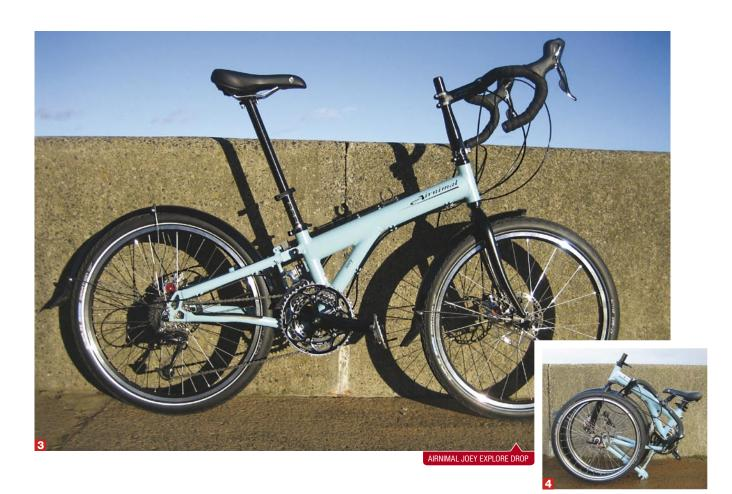
There are no hinges as such; the non-suspended rear triangle pivots underneath and other parts detach. To begin, you telescope the upper seat post into the lower post. Then you remove the front wheel.
