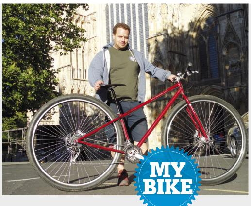
(Left) Dylan with his prototype, which fits riders from 5ft 3in to 6ft 5in. Production versions are custom built for the rider. They won't fit riders smaller than that but can, of course, be designed for taller riders (Below) The prototype uses 48-hole tandem hubs laced to 36in rims designed for unicyclists
