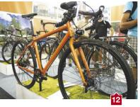
levers, hub dynamo lighting, and mounts for mudguards and disc brakes (hydraulic or mechanical). The show bike had a Gates CenterTrack Carbon belt drive. There is a chain-drive option, plus an urban version, The City 2. **en.tout-terrain.de**
