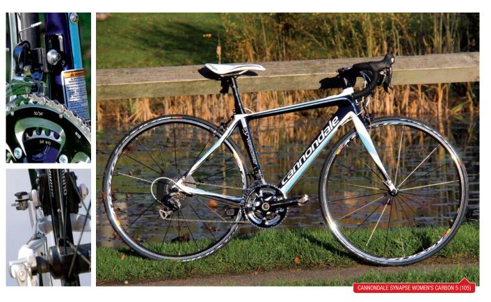
handlebar soon looked grubby. Shimano RS10s are a reliable choice thanks to straight pull spokes and an offset rear rim to reduce dish. They're shod with Schwalbe Lugano tyres, which rolled well enough and more smoothly than you'd expect from only 23mm, thanks to the frame.
