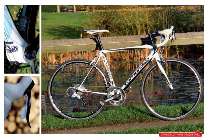
different properties, I think it does. It's not suspension as we know it, but it's probably worth one or two tyre sizes in terms of comfort on rough roads. Size for size, Synapse frames also have slightly taller head tubes and shorter top tubes, which facilitate a suitable position for long rides at less than eyeballs-out effort.
