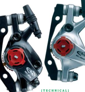
Avid's BB7 mechanical disc brake comes in two versions – road and mountain – with different cable pull
