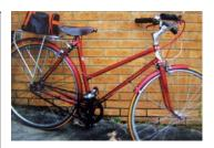
her a 1970 Coventry Eagle Elite, built from Reynolds 531 tubing, and upgraded it so that it weighs under 24lb, complete with mudguards, prop stand, rack, and 3-speed hub.
