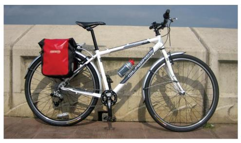
strengthen it here. The fork is rigid chrome-moly – a better and lighter option for any usage than a substandard suspension fork. A larger than normal offset (50mm) keeps the steering sharp and the front wheel further from your feet.
