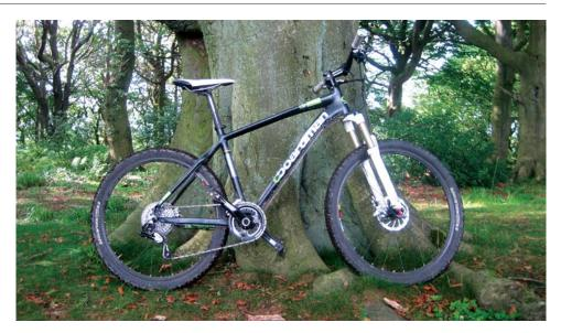
you can set the positive and negative air springs precisely to your weight and preference. Its tapered steerer means it has a bigger (1.5in) lower headset race, which should reduce steering flex and lengthen bearing life.
