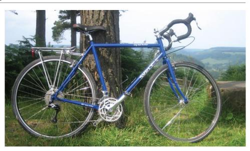
rather have 170mm, for while the LHT's low bottom bracket makes it easy to get a foot down, it can also result in pedal strikes on rougher tracks. And the LHT is a robust tourer that will readily tackle such terrain. A chainstay transfer reads: Fatties Fit Fine. Tyres, that is! There's just clearance for 50mm, even with mudguards.
