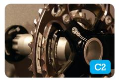
It's a new size for bottom brackets, with a 30mm tubular axle and larger bearings press-fitted into a 42mm internal diameter shell. The idea is to improve both stiffness and durability. You can expect to see a few of these bottom brackets on Cannondale bikes at Cycle, since they developed the idea, but BB30 is an open standard and FSA (pictured) were not the only crankset manufacturer to display bottom bracket models in this size at Eurobike.
