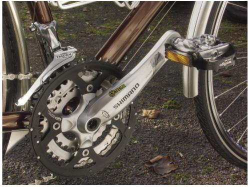
after I'd lowered it as close as possible to the chainset teeth. When the middle ring wears out a 37T replacement is likely to work a bit better, by exactly matching the intended middle-outer difference of this mech, which has a deep enough cage to allow a much smaller inner ring to be used – even 22T appears possible.
