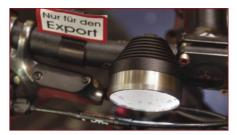
Major improvements in the efficiency of white LEDs were made during 2007. The latest emitters can now yield up to 90 lumens of light per electrical watt. That's three times the efficiency of the best halogen bulbs and 50% better than a HID lamp. Since LEDs also last a great deal longer than either of the above, and unlike them can be efficiently dimmed for further economy or to avoid causing dazzle, the road and trail ahead belongs to LEDs.
