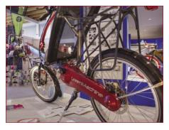
of their clean, green recumbent pedalling machine. A specially modified Rohloff hub provides an intermediate gearbox, coaxial with the rear suspension pivot and transferring chain drive from the right side to the left. A two-legged fork rather spoils the asymmetry, but a monoblade is in development. See www.flevobike.nl
