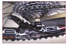
This 'shadow' design of low-profile mech is one of the options in the new XT groupset being rolled out during this year.
