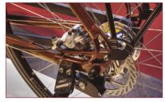
Of more immediate interest is this neat arrangement for mounting the disk brake, carrier and propstand on a production Cannondale trekking bike. Other manufacturers please take note.
