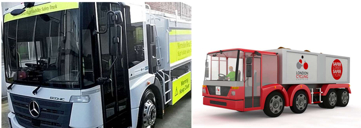
Figure 5 Examples of 'direct vision' cabs
